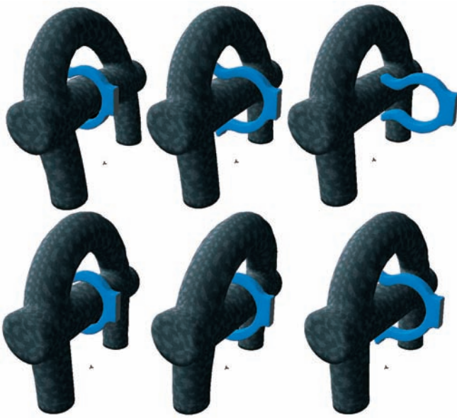
Fig. 16. Snapshots of the interactive snap-in and snap-out task on deformable pipes. At the top, the pushing phase of the snap-in task. At the bottom, the user withdraws the clip. This creates deformations of the pipes, especially if the friction coefficient is very large.
