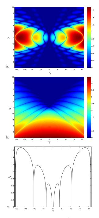
Fig. 2: (Color online) a. Growth rate  $\sigma'$  represented in the  $(\gamma,\alpha)$ -plane. b. Growth rate for the Mathieu equation in the  $(\gamma,\widetilde{\alpha})$ -plane. c. Both solutions are identical when  $\alpha=\widetilde{\alpha}=0$ .
