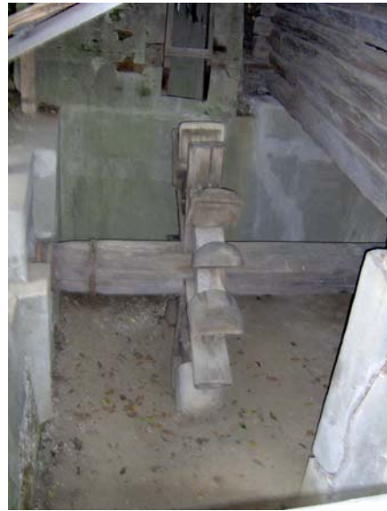
Figure 1. Wooden water wheels from the Village National Museum "Dimitrie Gusti" of Bucharest: (a) breastshot wheel; (b) vertical Norse wheel.
