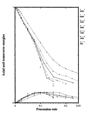
Figure 1. Variation with precession rate (pr between 0 and 0.25) of axial (lower curves) and transverse (upper curves) mean kinetic energies for different Reynolds numbers (between 500 and 5000). The energies are measured relatively to the solid body rotation energy
