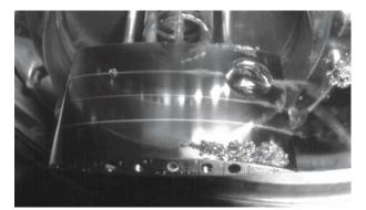
Figure 12. Growth of a nucleus on the suction side of a hydrofoil
