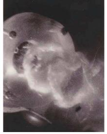
**Figure 23.** Cavitating vortex rings issuing from a StratoJet® self-resonating cavitating jet. Resonance is achieved through a feedback mechanism between the shear layer at the nozzle lip and the upstream organ pipe tube leading to the orifice. The frequency of emission of the rings is the same as the organ pipe frequency (Courtesy of Dr. Georges Chahine from Dynaflow, Inc.)
