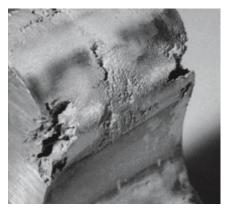
Figure 21. A typical example of cavitation erosion
