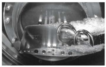
Figure 6. Two cavitation bubbles on the suction side of a hydrofoil
