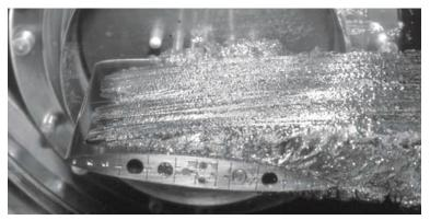
Figure 5. Supercavity flow around a hydrofoil in a cavitation tunnel
