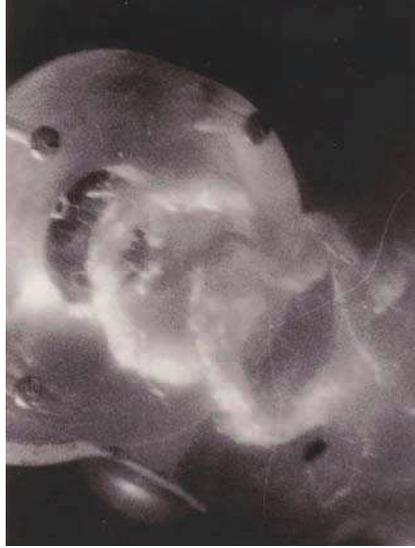
**Figure 23.** Cavitating vortex rings issuing from a StratoJet® self-resonating cavitating jet. Resonance is achieved through a feedback mechanism between the shear layer at the nozzle lip and the upstream organ pipe tube leading to the orifice. The frequency of emission of the rings is the same as the organ pipe frequency (Courtesy of Dr. Georges Chahine from Dynaflo, Inc.)
