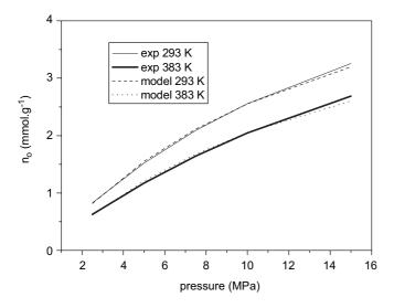
Fig. 2. Hydrogen adsorption isotherms: experiments vs. model.
