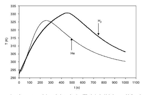
Fig. 8. Comparison of the experimental temperature evolution at the hottest location (T3) obtained with hydrogen and helium charging with an initial flow rate regulated at  $3.53 \times 10^{-4} \, \mathrm{m}^3 \, \mathrm{s}^{-1}$ .
