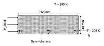
Fig. 9. Sketch of the simulated tank showing the boundary conditions.
