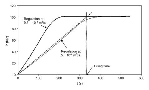
Fig. 5. Experimental pressure profiles for two different initial flow rates of hydrogen.
