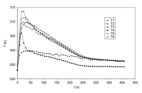
Fig. 7. Temperature histories without adsorbent material (empty tank) for a charge pressure of 10 MPa and with a flow rate regulated at  $9.5 \times 10^{-4} \, \text{m}^3 \, \text{s}^{-1}$ .
