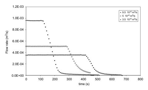
Fig. 3. Typical flow rate profiles at different regulation values with hydrogen.
