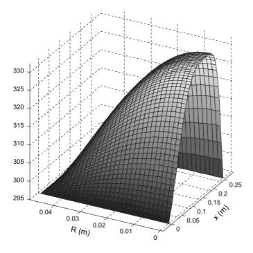
Fig. 11. Surface of hydrogen temperature in the tank at time  $t = 360 \,\mathrm{s}$ .
