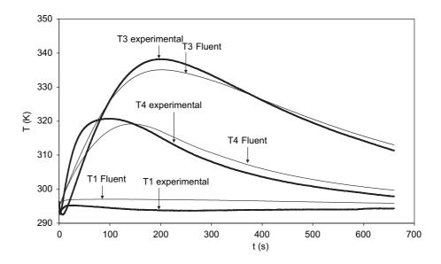
Fig. 10. Comparison of the experimental and numerical temperature profiles at different locations in the tank for an initial flow rate equal to  $9.5 \times 10^{-4} \, \mathrm{m}^3 \, \mathrm{s}^{-1}$  and a final pressure of  $10 \, \mathrm{Mpa}$ .
