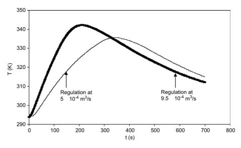
Fig. 6. Effect of the initial flow rate on the experimental temperature evolution at the hottest location (T3) for the case of hydrogen.
