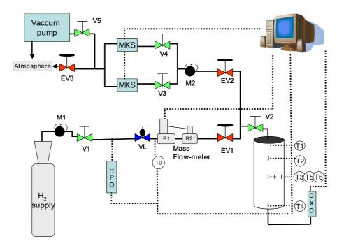
Fig. 1. Experimental setup for hydrogen storage.
