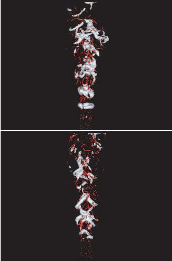
Fig. 17. LES of the natural jet at Re = 25\,000 : instantaneous visualizations at two different times. White: low pressure isosurface; dark: regions of Q > 0 (courtesy Silva).
