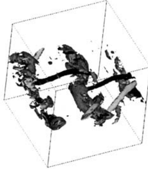
Fig. 14. Comparison of various SGS models (Smagorinsky, Structure-Function, Plateau-Peak, FSF, SSF) applied to a temporal mixing layer, visualized by iso-surfaces \omega_x = \omega_i (black), \omega_x = -\omega_i (light grey) and \omega_z = \omega_i = -2U/\delta_i (dark grey).
