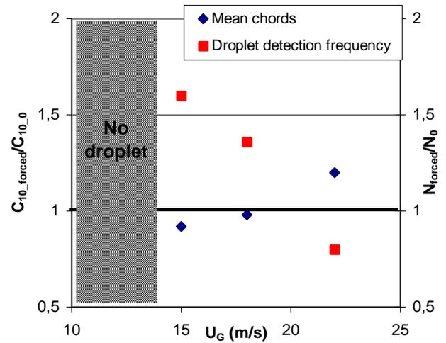
**Figure 14 – Optical probe measurements for a forcing at a transverse wavelength adapted to each gas velocity, for  $M=16$ . Comparison of the ratio of mean chord in forced case to mean chord in unforced case (blue symbols) ; ratio of droplet detection frequency in forced case to unforced cases (red symbols).**
