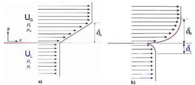
Figure 5 – Raynal's linear stability (a) and real (b) inlet velocity profiles
