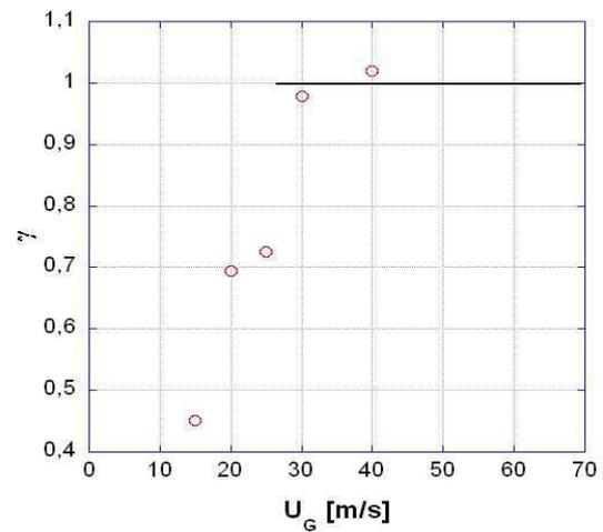
Figure 10 - Dimensionless ligaments lineic density as a function of the gas velocity,  $M=16$  (Rayana et al 2006)
