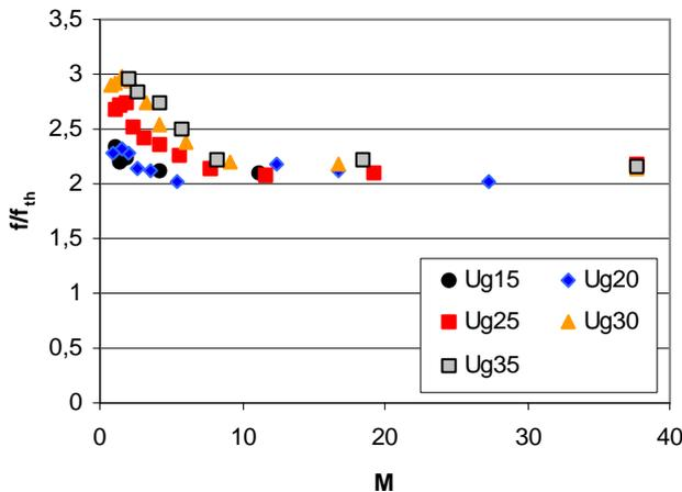
Figure 7 – Ration of measured axial and theoretical frequency as a function of  $M$ . Experimental data is well captured by theory for large  $M$ .
