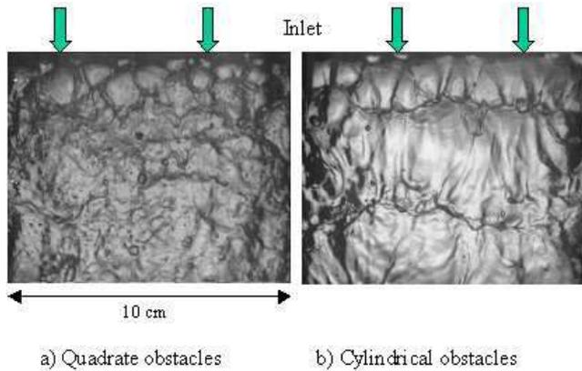
**Figure 12 – Large obstacles (characteristic length 4mm)  $U_G=18m/s$ ,  $M=16$ .**
