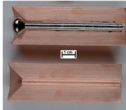
FIG. 2: Typical rods produced in the copper mould.
