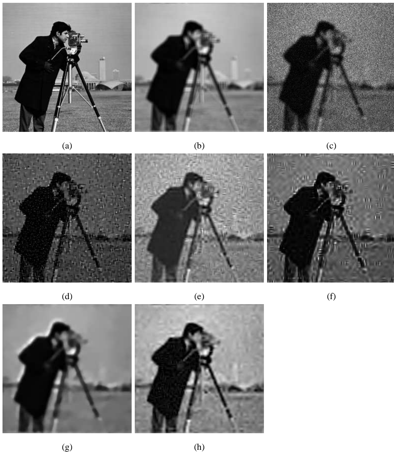
Figure 4. Deconvolution of the cameraman ( \text{Intensity} \leq 30 ). (a) Original, (b) Blurred, (c) Blurred&noisy, (d) RL-TV [7], (e) NaiveGauss [12], (f) RL-MRS [3], (g) FTITPR [55], (h) Our Algorithm.
