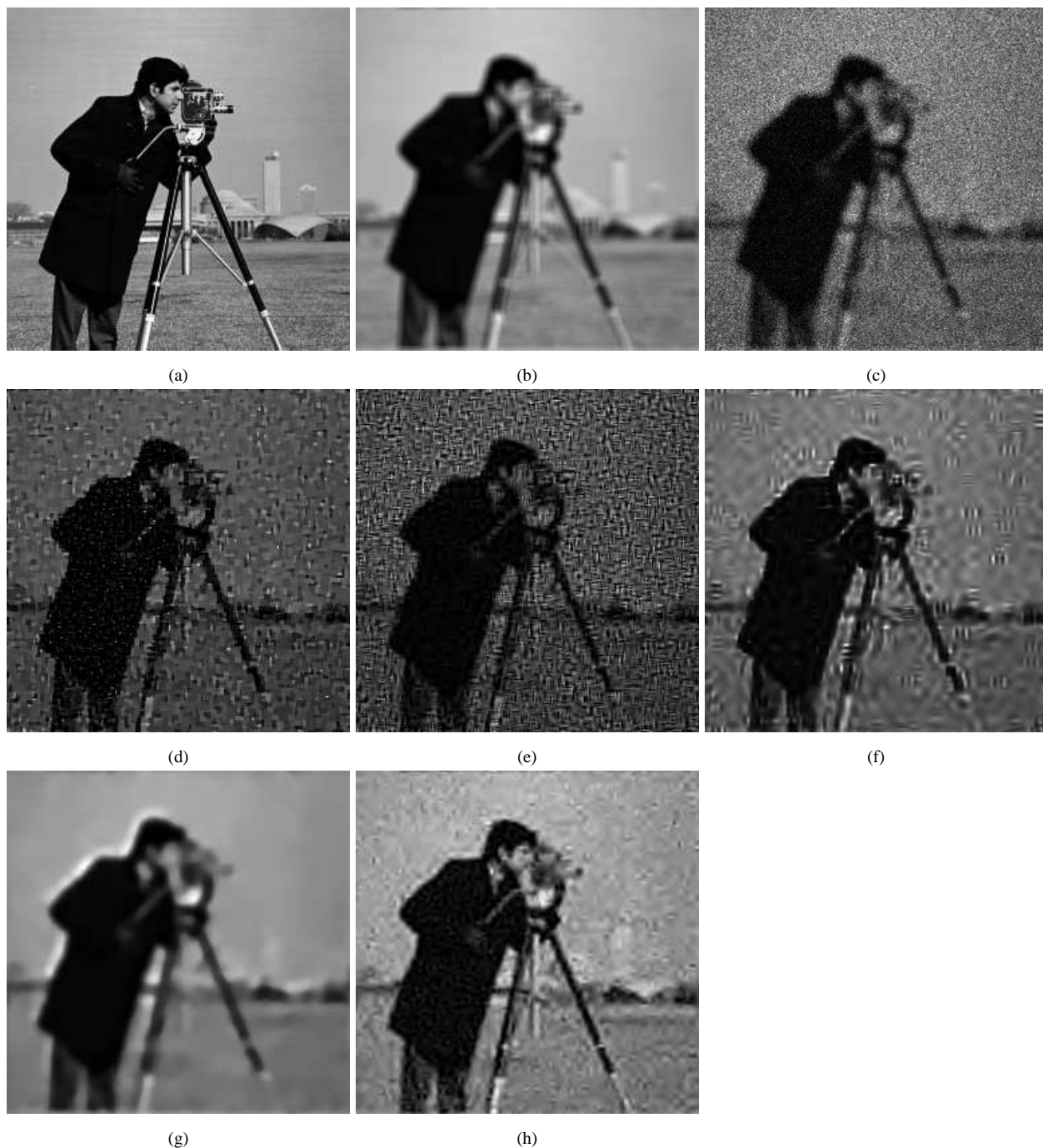
Figure 4. Deconvolution of the cameraman (Intensity \leq 30 ). (a) Original, (b) Blurred, (c) Blurred&noisy, (d) RL-TV [7], (e) NaiveGauss [12], (f) RL-MRS [3], (g) FTITPR [36], (h) Our Algorithm.
