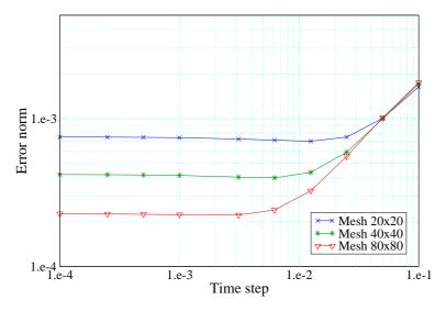
FIGURE 4. Error for the gas mass fraction at t = 0.5, as a function of the time step (discrete  $L^2$  norm).
