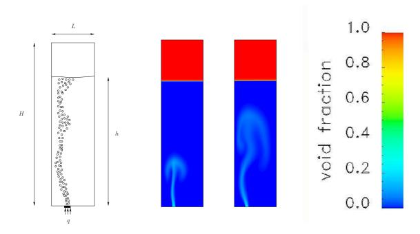
FIGURE 8. Bubble column: geometry of the problem and void fraction at times 2s, 4s and 40s.
