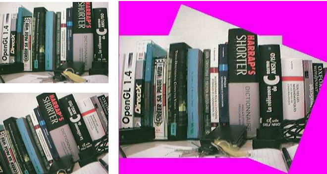
Fig. 3. Result of three-layer blending: left, top and bottom the original images, right the mosaic.
