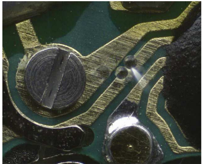
Fig. 6. A snapshot from the virtual microimager: a tip is manipulated polystyrene balls of diameter 250\mu\text{m} .
