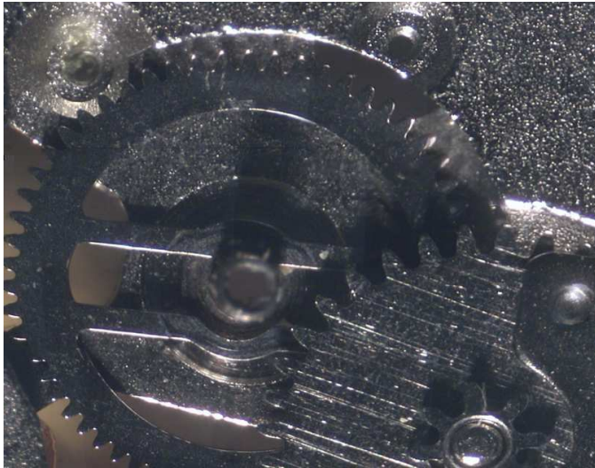
Fig. 5. Mosaicing of a watch gear: 25 images, 1934 \times 1516 pixels, 3\mu\text{m}/\text{pixel} , 26\text{mm}^2 and 7 Mo.
