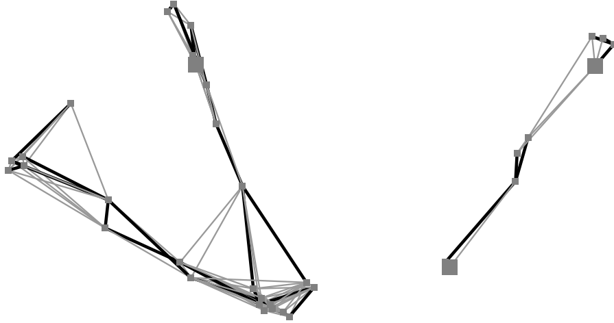
Fig. 4. A graphical view of a MANET. Black thick links are colored by the Spanning Forest Algorithm and belong to the forest. Bigger nodes are the ones owning a token , they are the roots or the spanning trees.
