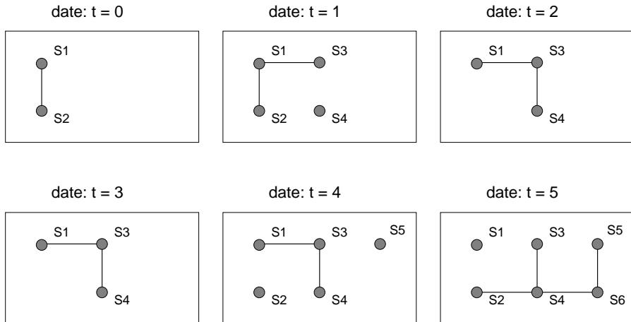
**Fig. 2.** Snapshots of a Dynamic Graph on the time interval  $[0, 5]$ . During a period of time the graph may not change as it is the case during interval  $[2, 3]$ . Some vertices may appear and disappear and appear again, as illustrated by vertex  $s_2$ .
