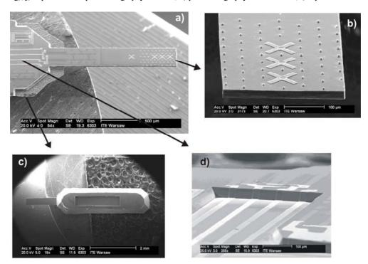
Fig. 2: SEM image of the force sensor: a) front side of the sensor with piezoresitive cantilever, b) end of the cantilever (gripping area), c) backside cavity, d) front-side depression for pads.
