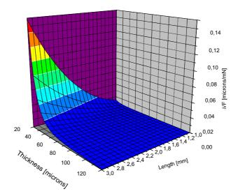
Fig. 3: Scaling of a silicon force sensor with a d/F ratio depending on thickness t and length L. Width of the silicon beam is 350 microns.
