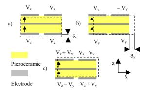
Fig 4: Working principle of the MOC with z-, y-mode and coupled y-z-mode. All three modes can be used for manipulation tasks.
