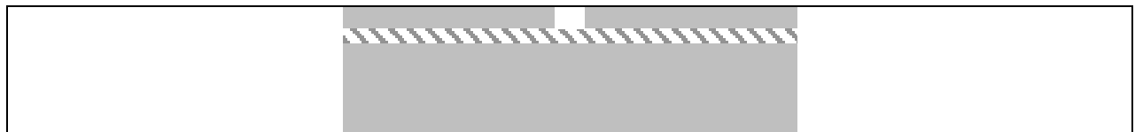
Fig.3. Patterning within the "active" SOI wafer of the cavity underneath the hot wire anemometer.
