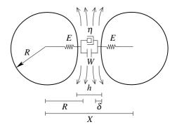
FIG. 1: Sketch of normal particle interaction. A force between elastic surfaces (modulus E) is transmitted partly through the fluid (visosity  $\eta$ ) and partly through possible remote interaction (labeled *W*). It can deform them (deflection  $\delta$ ), which affects the flow. The consequence is that the center-to-center distance X and the gap h between both surfaces exhibit two distinct dynamics.
