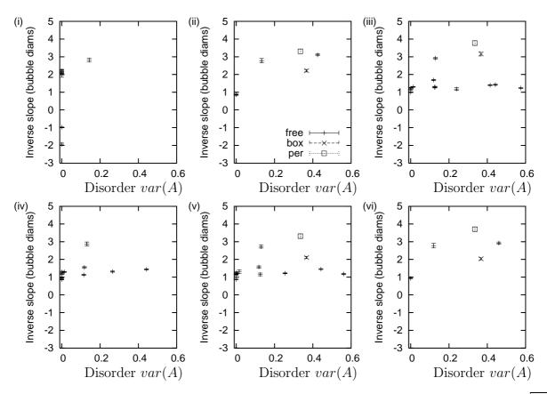
Figure 8: Screening length  $\ell_s$  of  $std(\Delta p)$  (eq. 3), in units of bubble diameter  $D=2\sqrt{\langle A\rangle/\pi}$ , after (i) inflation (ii) an edge stretch, (iii) a T1, (iv) a T2, (v) coalescence, and (vi) division.
