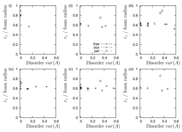
Figure 9: Cross-over radius  $r_c$ , in units of foam radius, after (i) inflation, (ii) an edge stretch, (iii) a T1, (iv) a T2, (v) coalescence, and (vi) division. It is rarely possible to measure it for bubble inflation.
