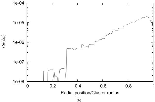
Figure 11: The effect on the bubble pressures of a 20% inflation event in a monodisperse ordered cluster of 1261 bubbles. In contrast to other perturbations to a monodisperse foam, and inflation events in disordered foams, there is no pressure screening: the pressure difference increases slightly towards the outside of the cluster. Note the scale, orders of magnitude smaller than figure 7.
