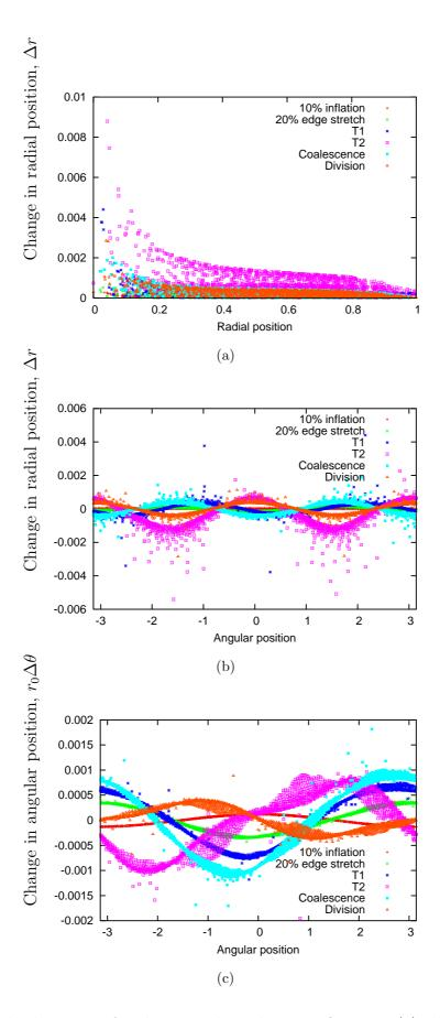
Figure 4: Bubble displacement, for the same data shown in figure 3. (a) The magnitude of the radial displacement as a function of radial position. (b) The radial displacement as a function of angular position. (c) The angular displacement as a function of angular position.
