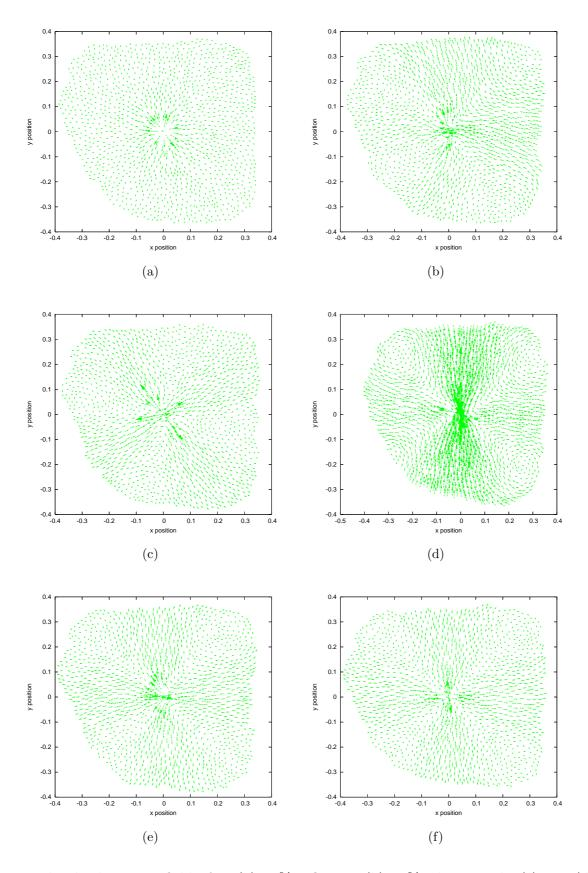
Figure 3: The displacement field after (a) 10% inflation, (b) 20% edge stretch, (c) T1, (d) T2, (e) coalescence, and (f) division, in a cluster of 1400 bubbles with  $var(A) \approx 0.12$ . The average displacement and rotation has been subtracted in each case, and the vector length multiplied by a factor of 200 (in a), 100 (in b) or 30 (in c,d,e,f).
