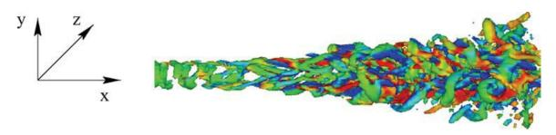
Figure 4. Isosurfaces of positive Q (green) and longitudinal vorticity (red and blue) for the supersonic jet at M = 1.4 and  $Re = 36\,000$ . The threshold is  $0.20(U_1/D)^2$ .
