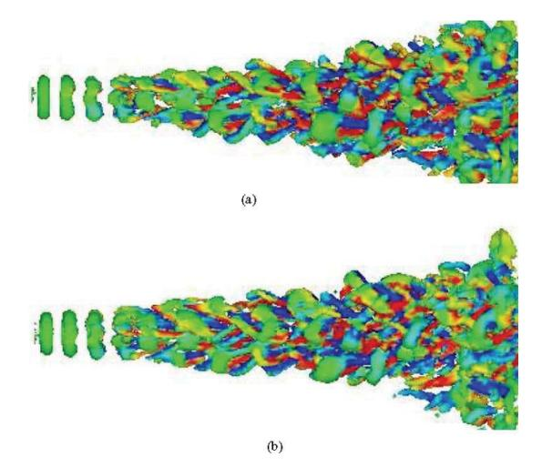
Figure 8. Isosurfaces of positive Q (green) coloured by the streamwise vorticity  $\Omega_x$  (red and blue) for the simulation LES<sub>for1</sub>. The threshold is  $0.20(U_1/D)^2$ . (a) View in bifurcating plane, (b) view in bisecting plane.
