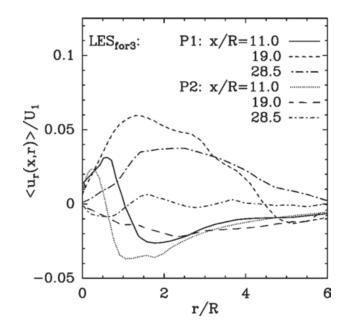
Figure 15. Bifurcating and bisecting profiles of the mean radial velocity for the simulation LES<sub>for3</sub>.  $P_1$  and  $P_2$  represent the bifurcating and bisecting planes, respectively.
