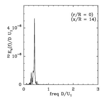
Figure 6. Temporal spectra of the streamwise velocity for the natural jet at M = 1.4 and  $Re = 36\,000$ .
