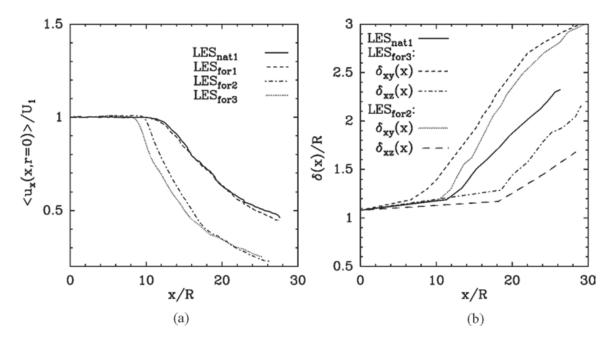
Figure 16. (a) Streamwise evolution of the mean centerline velocity for the LES<sub>for1</sub>, LES<sub>for2</sub> and LES<sub>for3</sub> simulations; (b) downstream evolution of the bifurcating and bisecting shear-layer thicknesses for the LES<sub>for2</sub> and LES<sub>for3</sub> simulations. The profiles for the natural jet are also given for comparaison.
