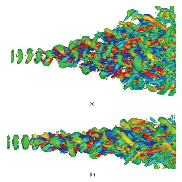
Figure 14. Isosurfaces of positive Q (green) coloured by the streamwise vorticity  $\Omega_x$  (red and blue) for the simulation LES<sub>for3</sub>. The threshold is  $0.20(U_1/D)^2$ . (a) View in bifurcating plane; (b) view in bisecting plane. The figure corresponds to animation 1.
