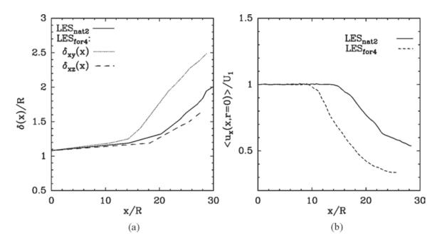
Figure 18. (a) Downstream evolution of the bifurcating and bisecting shear-layer thicknesses for the simulation  $LES_{for4}$ , (b) streamwise evolution of the mean centerline velocity for the simulation  $LES_{for4}$ . The profiles for the natural jet are also given for comparison.
