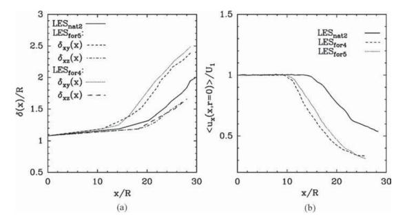
Figure 20. (a) Downstream evolution of the bifurcating and bisecting shear-layer thicknesses for the LES<sub>for4</sub> and LES<sub>for5</sub> simulations, (b) streamwise evolution of the mean centerline velocity for the LES<sub>for4</sub> and LES<sub>for5</sub> simulations. The profiles for the natural jet are also given for comparison.
