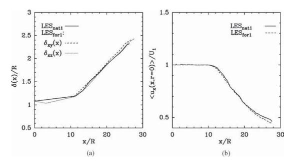
Figure 10. (a) Downstream evolution of the bifurcating and bisecting shear-layer thicknesses ( $\delta_{xy}(x)$  and  $\delta_{xz}(x)$ ) for the LES<sub>for1</sub> simulation; (b) streamwise evolution of the mean centerline velocity. The profiles for the natural jet are also given for comparison.
