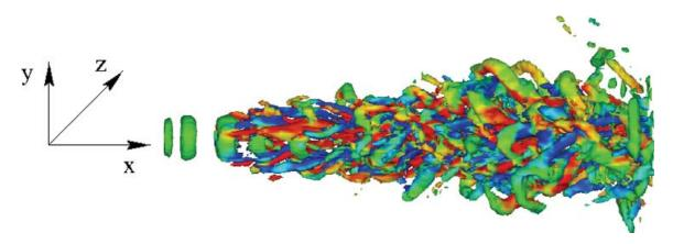
Figure 1. Isosurfaces of positive Q (in green) coloured by the streamwise vorticity  $\Omega_x$  (positive, red; negative, blue) for the subsonic jet at M = 0.7 and  $Re = 36\,000$ . The threshold is  $0.20(U_1/D)^2$ .
