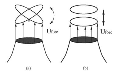
Figure 7. (a) Sketch of the flapping excitation, (b) sketch of the varicose excitation.
