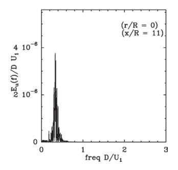
Figure 3. Temporal spectra of the streamwise velocity for the natural jet at M = 0.7 and  $Re = 36\,000$ .
