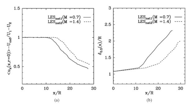
Figure 5. (a) Streamwise evolution of the centerline velocity decay, (b) streamwise evolution of the shear-layer thickness.  $U_{cof}$  is the local coflow velocity.
