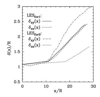
Figure 12. Downstream evolution of the bifurcating and bisecting shear-layer thicknesses ( $\delta_{xy}(x)$  and  $\delta_{xz}(x)$ ) for the LES<sub>for1</sub> and LES<sub>for2</sub> simulations.
