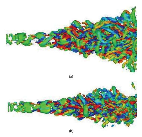
Figure 21. Isosurfaces of positive Q (green) coloured by the streamwise vorticity  $\Omega_x$  (red and blue) for the simulation LES<sub>for6</sub>. The threshold is  $0.20(U_1/D)^2$ . (a) View in bifurcating plane, (b) view in bisecting plane. The figure corresponds to animation 2.
