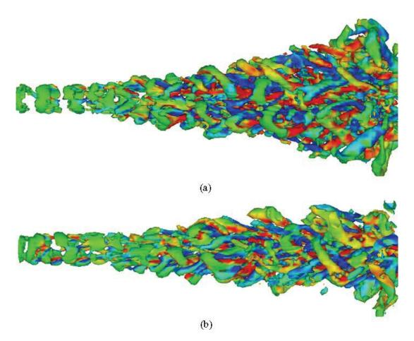
Figure 19. Isosurfaces of positive Q (green) coloured by the streamwise vorticity  $\Omega_x$  (red and blue) for the simulation LES<sub>for5</sub>. The threshold is  $0.20(U_1/D)^2$ . (a) View in bifurcating plane, (b) view in bisecting plane.
