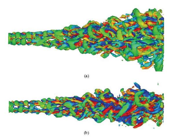
Figure 17. Isosurfaces of positive Q (green) coloured by the streamwise vorticity  $\Omega_x$  (red and blue) for the simulation LES<sub>for4</sub>. The threshold is  $0.20(U_1/D)^2$ . (a) View in bifurcating plane, (b) view in bisecting plane.
