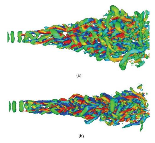
Figure 11. Isosurfaces of positive Q (green) coloured by the streamwise vorticity  $\Omega_x$  (red and blue) for the simulation LES<sub>for2</sub>. The threshold is  $0.20(U_1/D)^2$ . (a) View in bifurcating plane, (b) view in bisecting plane.
