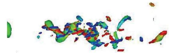
Figure 9. Isosurfaces of low pressure coloured by the streamwise vorticity  $\Omega_x$  for the simulation LES<sub>for1</sub>. The threshold is  $(p - p_0) = -0.05\rho_0 U_1^2$ .
