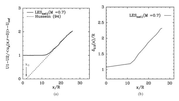
Figure 2. (a) Streamwise evolution of the centerline velocity decay, (b) streamwise evolution of the jet half-width.  $U_{cof}$  is the local coflow velocity and  $x_o$  is the virtual origin.
