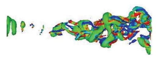
Figure 13. Isosurfaces of low pressure coloured by the streamwise vorticity  $\Omega_x$  for the simulation LES<sub>for2</sub>. The threshold is  $(p - p_0) = -0.05\rho_0 U_1^2$ .
