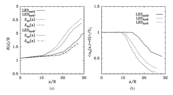
Figure 22. (a) Downstream evolution of the bifurcating and bisecting shear-layer thicknesses for the  $LES_{for5}$  and  $LES_{for6}$  simulations, (b) streamwise evolution of the mean centerline velocity for the  $LES_{for5}$  and  $LES_{for6}$  simulations. The profiles for the natural jet are also given for comparaison.
