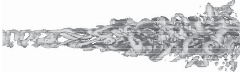
Figure 5. Isosurfaces of positive Q (green) and longitudinal vorticity (red and blue) for the supersonic jet at M = 1.4 and Re = 36\,000 . The threshold is 0.20(U_1/D)^2 . The figure corresponds to animation 2.
