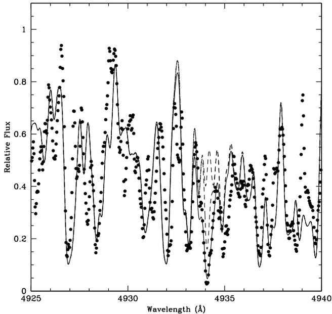
**Fig. 2.** Synthetic fit to the spectrum of ALW-C6 in the region of the Ba II line at  $\lambda 4934 \text{ \AA}$ . Black dots represent the observed spectrum. Lines are synthetic spectra for different  $[\text{Ba}/\text{M}]$  ratios: no Ba and +0.0 (dashed lines), +2.0 (best fit, continuous line).
