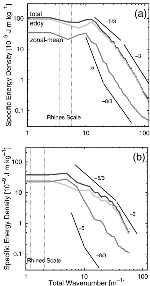
**Figure 4.** Kinetic energy spectra in total wave number ( $2\pi/\text{wavelength}$ ) for (a) the sloping bottom experiment and (b) the flat bottom case. The Rhines wave numbers for the max/min topographic  $\beta$  are marked by vertical lines. The solid straight lines are references for the slopes, and the  $-5$  line is the theoretical prediction by Sukoriansky et al. [2002] with  $C_z = 0.5$ .
