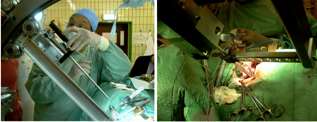
Figure 11: in vivo tests: instrument unplugged (left), umbrella deployed in the atrium (right).
