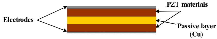
Fig. 3: Bending cantilever structure.
