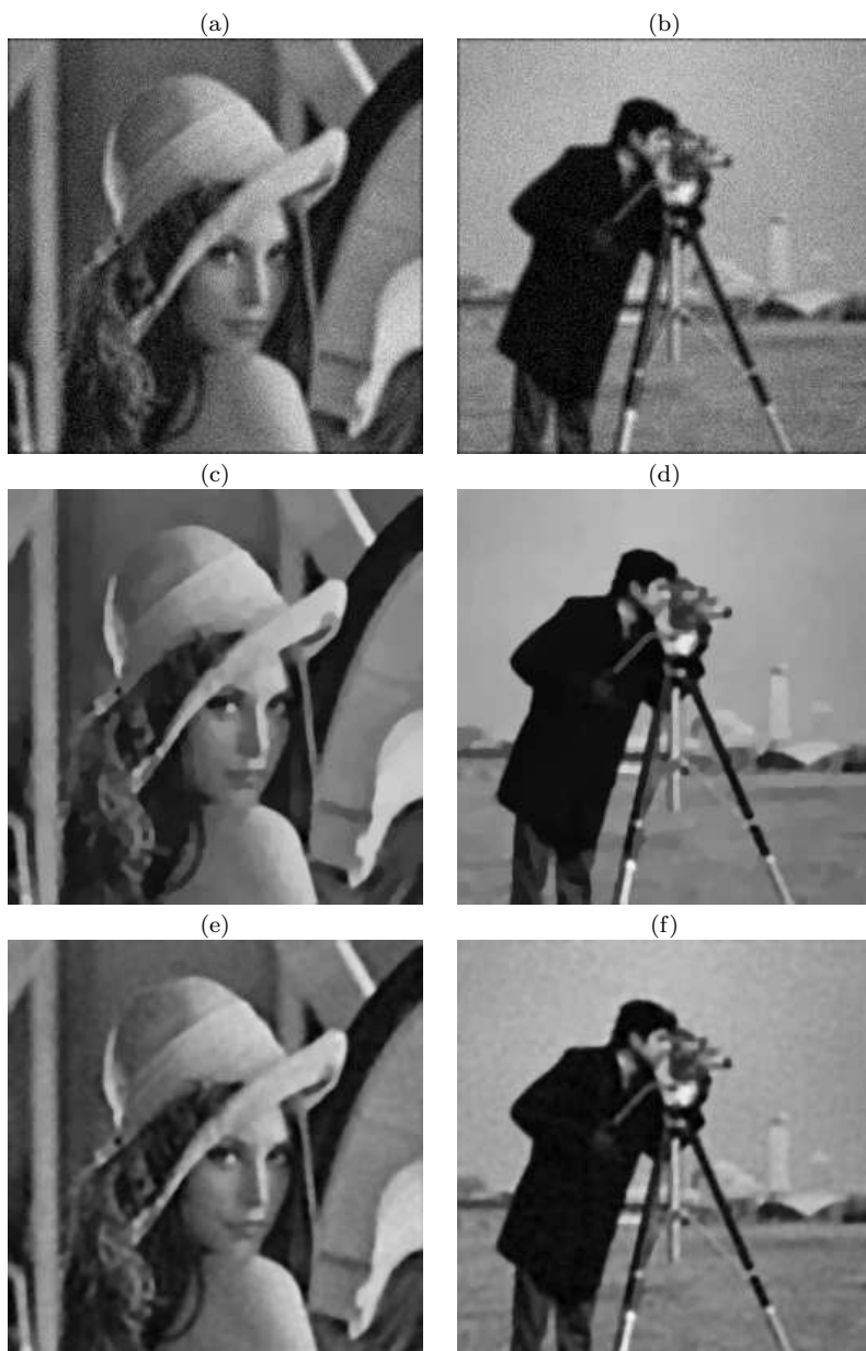
Figure 3: (a) and (b) : degraded images (convolved with a Gaussian kernel with standard deviation \eta = 5 , and then degraded by a zero mean Gaussian noise with standard deviation \sigma = 10 ), the original images are on top row of Figure 1; (c) and (d) : total variation restoration with schemes (75) and (24), with \lambda = 5 ; (e) and (f) : smoothed total variation based restoration with schemes (75) and (43), with \lambda = 5 and \beta = 10 .
