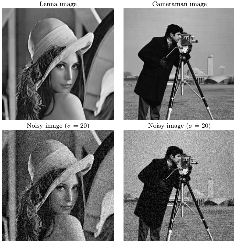
Figure 1: The classical Lenna and cameraman image, and their noisy version (additive zero mean Gaussian noise with standard deviation \sigma = 20 ).
