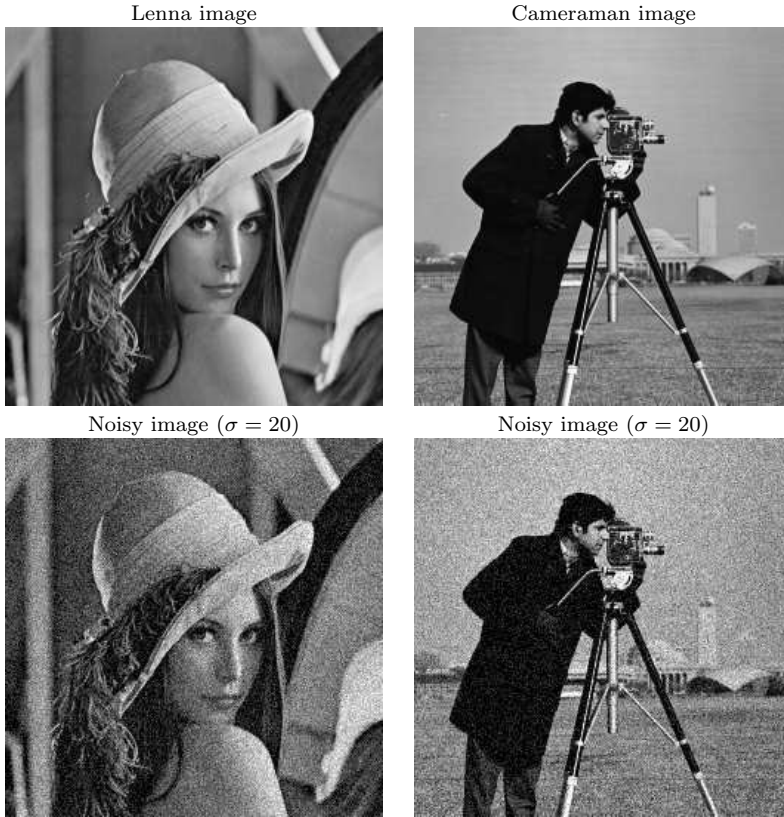
FIG. 3.1. The classical Lenna and cameraman image, and their noisy version (additive zero mean gaussian noise with standard deviation \sigma = 20 ).
