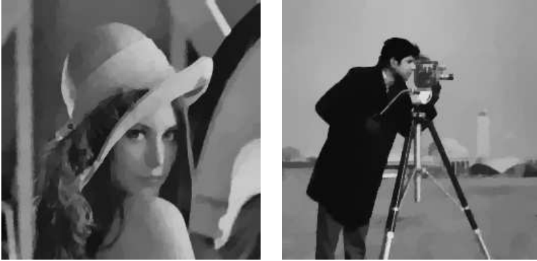
FIG. 3.2. Total variation restoration of the noisy images presented on the bottom row of Figure 3.1 with scheme (3.13). In both cases, the Lagrange multiplier is \mu = 30 .
