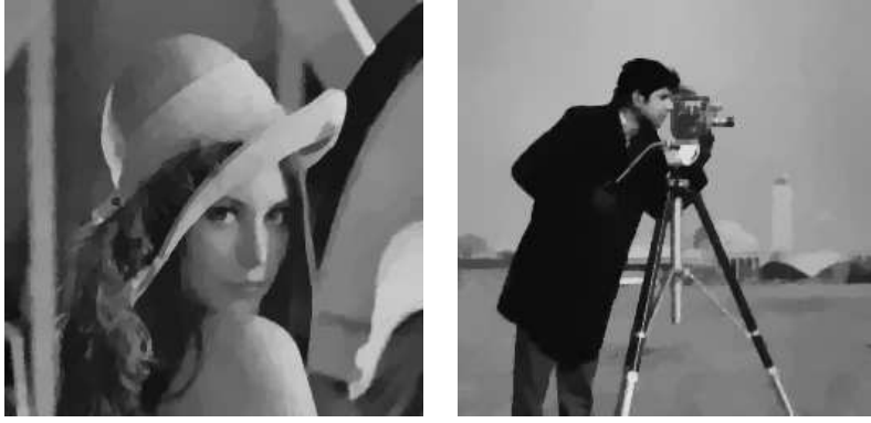
Figure 2: Total variation restoration of the noisy images presented on the bottom row of Figure 1 with scheme (24). In both cases, the Lagrange multiplier is \mu = 30 .
