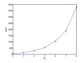
Figure 15: Number of MVPs with respect to  $M_x = \sqrt{M}$  (setting  $M_y = M_x$ ): rectangular lattice configuration with ka = 50 and  $b_x = b_y = 3$ . The GMRES(50) solver is used fixing  $tol = 10^{-8}$  (Dirichlet problem).
