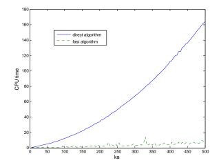
Figure 9: Comparison of the CPU time for computing one MVP using the direct and fast algorithms. We take: ka = 100,  $b_x = 3$  for the single-row configuration (Dirichlet problem).
