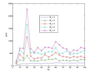
Figure 14: Number of MVPs with respect to the wavenumber ka: rectangular lattice configurations with  $M_x = 5$ ,  $M_y = 2, ..., 6$ . We consider  $b_x = b_y = 3$  and solve the linear system using the GMRES(50) solver for  $tol = 10^{-8}$  (Dirichlet problem).
