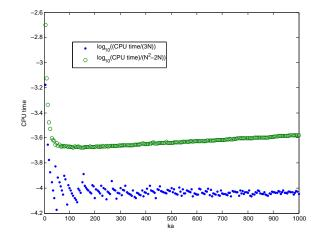
Figure 5: Behaviour of the CPU time according to the wavenumber  $ka_p$  for building the matrix  $\mathcal{A}$  in the case of the scattering by two circular cylinders fixing  $N_p$  by formula (21).
