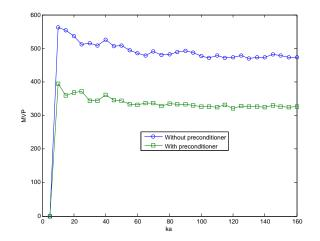
Figure 18: Number of MVPs with respect to the wavenumber ka for a unstructured configuration (with and without preconditioner).
