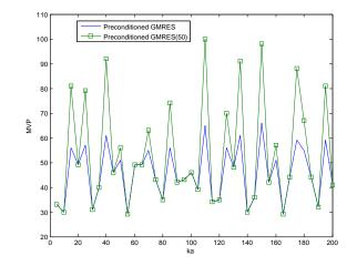
Figure 16: Number of MVPs with respect to the wavenumber ka for the single-row configuration with M = 75 and  $b_x = 3$ . The solution is obtained with the preconditioned GMRES and GMRES(50) for  $tol = 10^{-10}$  (Dirichlet problem).
