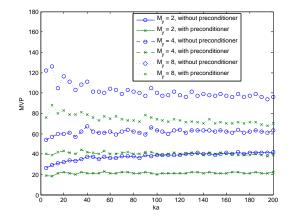
Figure 13: Number of MVPs with respect to the wavenumber ka for the rectangular lattice configuration with  $b_x = 8$  and  $b_y = 13$ . We fix  $M_x = 8$  and  $M_y = 2, 4, 8$ . The solution is obtained without and with the preconditioned GMRES(50) for  $tol = 10^{-8}$  (Dirichlet problem).
