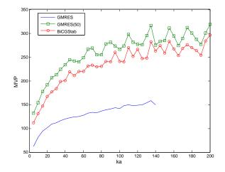
Figure 10: Number of MVPs with respect to the wavenumber ka: single-row configuration with 75 obstacles and  $b_x = 3$ . We use different iterative solvers: GMRES, GMRES(50) and BiCGStab. The tolerance is  $tol = 10^{-10}$  (Dirichlet problem).
