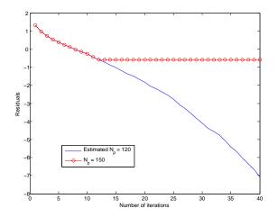
Figure 7: Evolution of the residuals with respect to  $n^{iter}$  for  $N_p = 120$  and  $N_p = 150$ .
