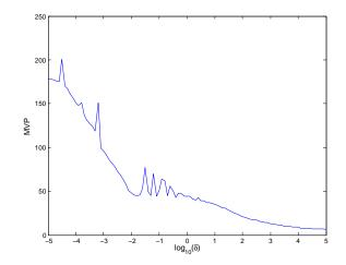
Figure 12: Number of MVPs with respect to the distance  $\delta$  between two obstacles. We fix: ka = 100, M = 10 obstacles. The solution is obtained with GMRES(50) for  $tol = 10^{-8}$  (Dirichlet problem).
