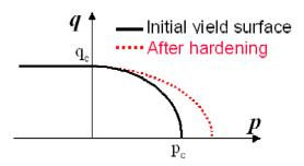
Fig. 1. The proposed yield criterion for amorphous silica
