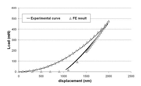
Fig. 6. Nanoindentation experimental and numerical load-penetration curves
