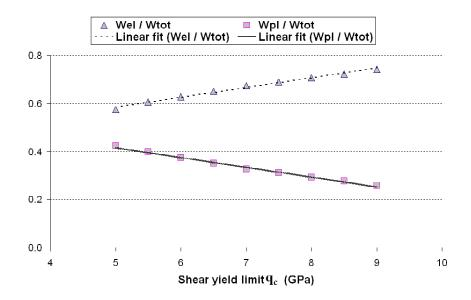
Fig. 5. FE analysis of the dependence of  $W_{el}/W_{tot}$  and  $W_{pl}/W_{tot}$  on shear yield limit  $q_c$ . The experimental values of  $W_{pl}/W_{tot}$  and  $W_{el}/W_{tot}$  are respectively 0.33  $\pm 0.01$  and 0.67  $\pm 0.01$ .
