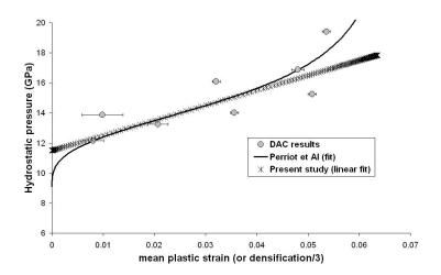
Fig. 2. Densification-induced hardening obtained from DAC experiments (extracted from Perriot [24]) and the linear law used in this paper
