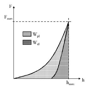
Fig. 4. Definition of the plastically dissipated energy  $W_{pl}$  and the elastically restored energy  $W_{el}$  from a typical load-penetration curve
