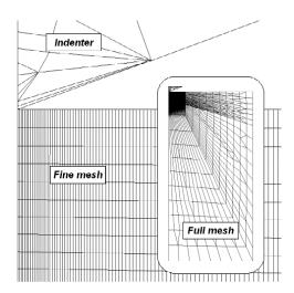
Fig. 3. FE mesh used for the modelling of the cone indentation test
