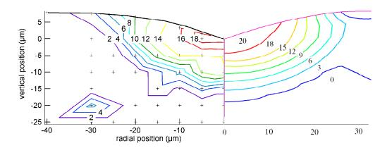
$Fig.\ 7.\ Densification\ map,\ \text{-left}: experimental\ results,\ \text{-right}: finite\ element\ results$
