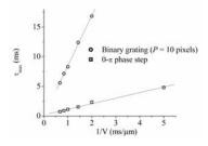
**Figure 6** Cross correlation functions obtained with two observation volumes, far apart by 8.5  $\mu$ m, produced with a binary phase grating of half period P=10 pixels on the spatial light modulator. The fluorescent entities are 20 nm beads and the velocity of the flow is 1.5, 1.2, 1, 0.7 and 0.5  $\mu$ m/ms. Error bars are standard errors of the mean.
