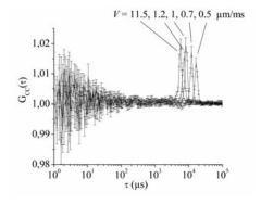
**Figure 7** Cross correlation functions obtained with two observation volumes, far apart by 1.27, 1.97 and 2.8  $\mu$ m produced with a echelette grating of period P = 60, 45 and 30 pixels on the SLM. The flow speed is 1.5  $\mu$ m/ms and the solution is seeded with R6G molecule at a nM concentration. Error bars are standard errors of the mean.
