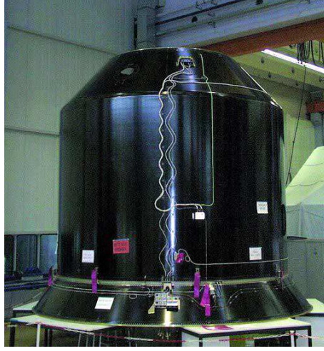
Fig. 4. The SYLDA5 satellite support
