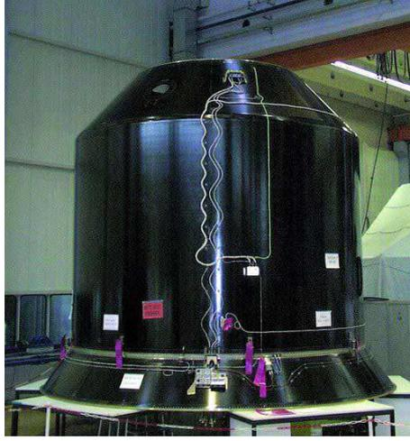
Fig. 4. The SYLDA5 satellite support
