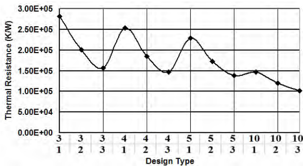
Fig. 8. Thermal resistance of the thermocouples implemented in the final mask. The two rows of numbers on the abscissa represent respectively the quantities a and b defined in the text.
