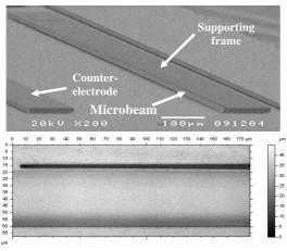
Figure 1: Microcantilever specimen in-plane bending
