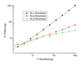
Figure 3: The numbers of required connection pads for 1D, 2D and 3D control circuit
