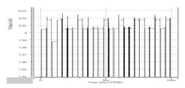
Figure 5: Transient simulation of the input and output signals of the level shift device
