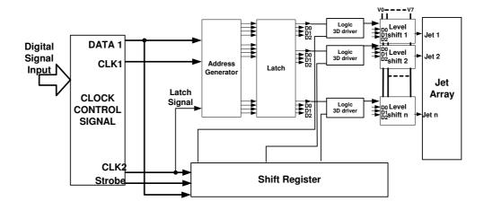
Figure 1: An inkjet print head digital driver block diagram
