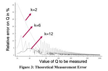
The ripples observed on the curves on figure 3 correspond to the fact that the final  $V_0/k$  value may not correspond exactly to a maximum of the decaying signal. The number of elapsed pseudo-periods is then an
