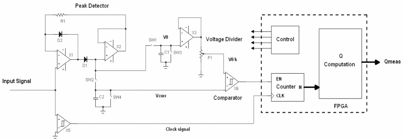
**Figure 4: Prototype architecture for step response measurement**
