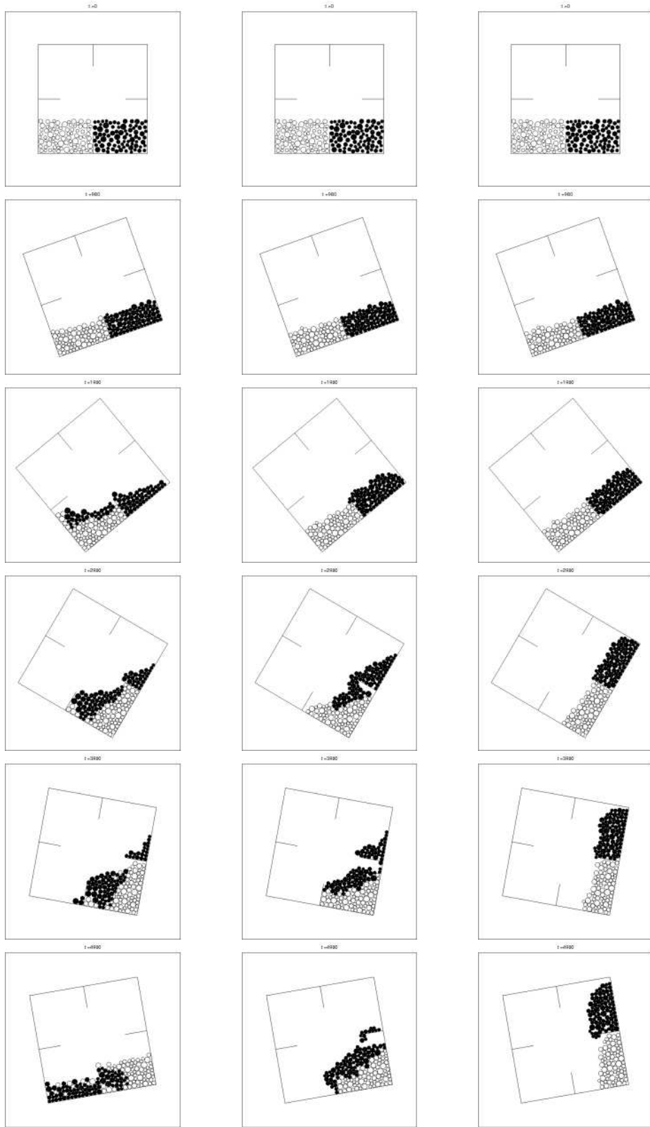
FIGURE 12. Gluey lotto: configurations at different time-steps for \gamma_{min} = 0 on the left (inelastic contacts), \gamma_{min} = -1 in the middle (gluey rough particles) and \gamma_{min} = -\infty on the right (gluey smooth particles).
