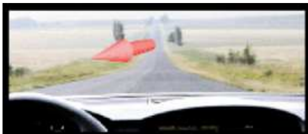
Figure 2: In-car Augmented Reality: Guiding driver's attention to dangerous situation. The arrow indicates the position of imminent danger (from [6]).
