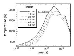
Fig. 6. Evolution of the lattice temperature versus time for various radial distances in bulk Co irradiated with Pb ions at room temperature as calculated using thermal spike simulations.  $T_m$  is the melting temperature of bulk Co.
