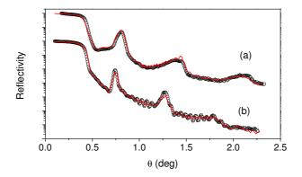
Fig. 2. Experimental and fitted x-ray reflectometry patterns of the (Tb-Fe 5 nm/Co 3 nm) multilayer: asdeposited (a) and irradiated with Pb ions at the fluence  $7 \times 10^{12}$  ion cm<sup>-2</sup> (b).
