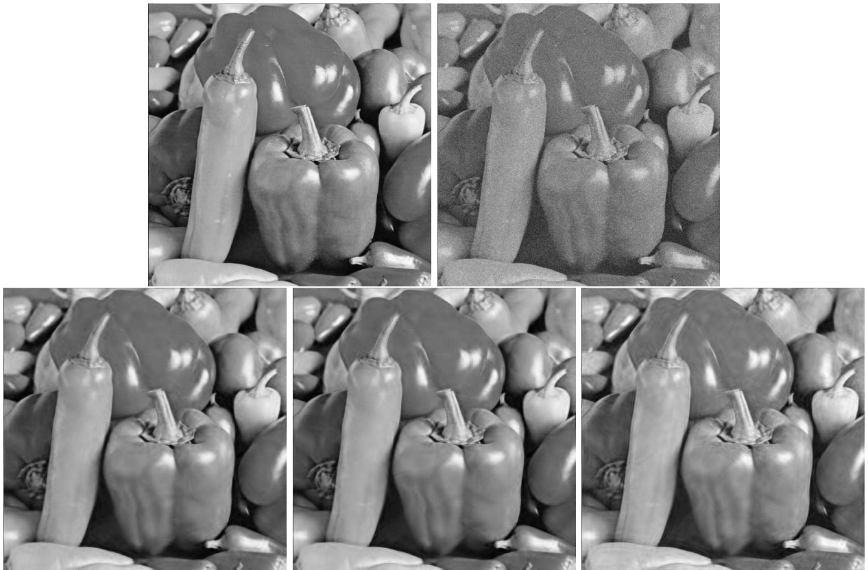
Figure 16: Comparison of denoising performance of several digital implementations of the curvelet transform. Top left: original image. Top right: noisy image \sigma = 20 . Bottom left: denoised with DCTG1 using the rectopolar DRT. Bottom middle: denoised with DCTG1 using the FSS DRT. Bottom right: denoised with DCTG2 using the wrapping implementation.
