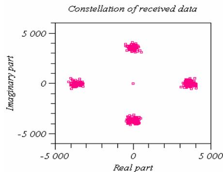
**Figure 3: Constellation of received data in TDD mode**
