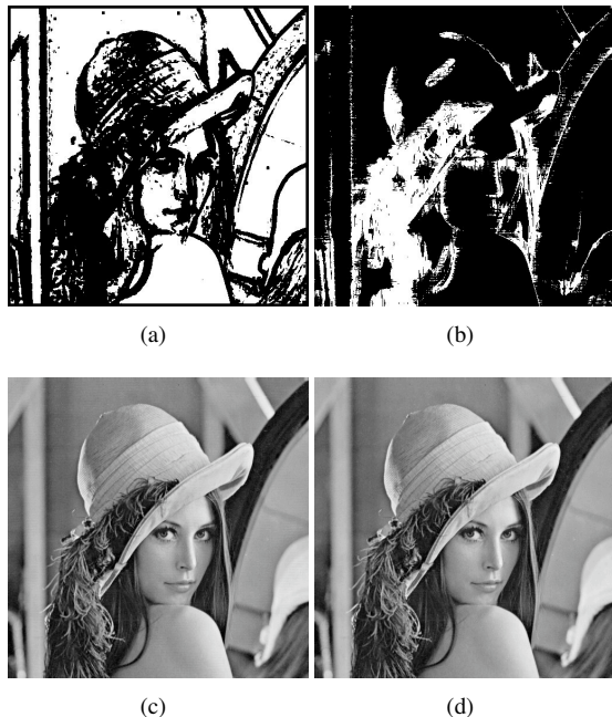
Figure 2. The two computed binary masks, i.e smooth areas, M_S (a), and textures M_T (b) along with the corresponding marked images (c) and (d).
