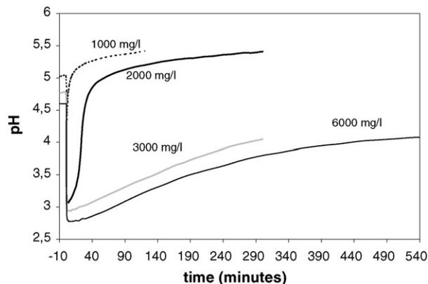
Fig. 2. Effect of Pb sorption on the pH of the solution for HAP<sub>2</sub>.
