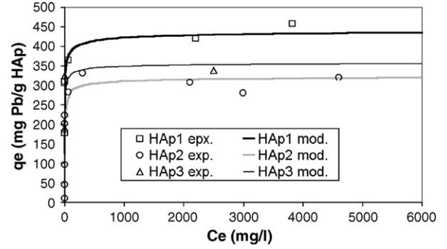
Fig. 5. Adsorption isotherms for the three hydroxyapatites.
