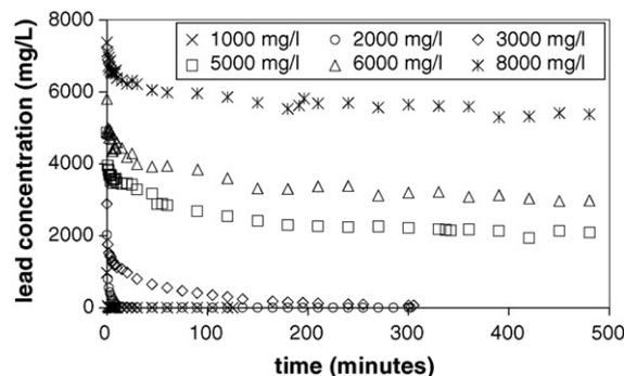
Fig. 1. Batch sorption kinetic measurements for HAP<sub>2</sub>.
