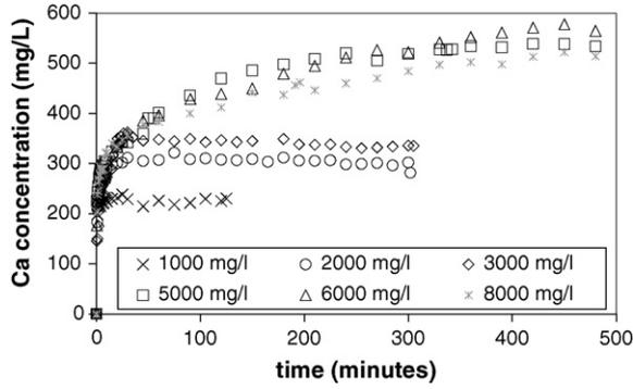
Fig. 3.  $\text{Ca}^{2+}$  released into the solution for HAp<sub>2</sub>.
