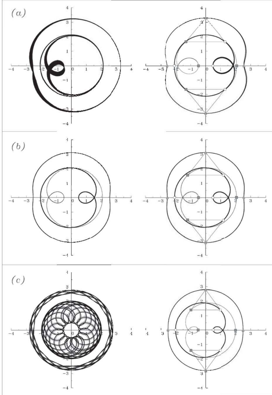
Fig. 16. Absolute trajectories of three vortices (left) and the respective choreographies (right) for motions of the type  $\{3\}$  at collinear initial state and the following parameter values:  $\mu = -1$ ,  $\gamma^2 L = -2$  and (a) —  $X_2^2 = 0.4811$ ,  $t = (-3.3750; 6.0000; 0.3750)$ ; (b) —  $X_2^2 = 0.4833$ ,  $t = (-3.7722; 6.4218; 0.3504)$ ; (c) —  $X_2^2 = 0.5$ ,  $t = (-4.7112; 7.4074; 0.3038)$ .
