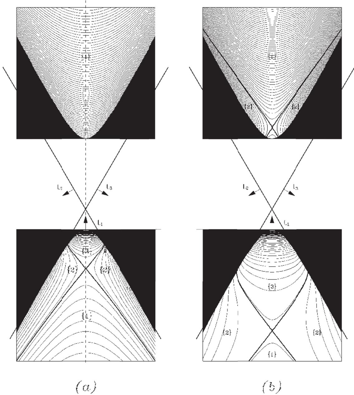
Fig. 3. Phase portraits of three-vortex problems in PR (2.13) at  $\mu = -1.5$  and  $L < 0$  — in the lower part,  $L > 0$  — in the upper part:  $\gamma^2|L| = 2$  — (a); in the lower part  $\gamma^2|L| = 0.65$  — (b). Figures mark the points in PR that correspond to the initial conditions for the experiments the results of which are given in figure 13.
