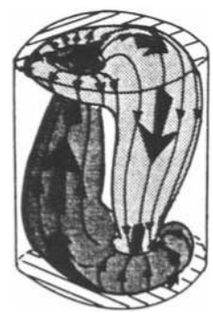
Fig.16. Schematic flow pattern for the asymmetric regime in a vertical cylinder heated from below. From Bontoux et al., 1986.
