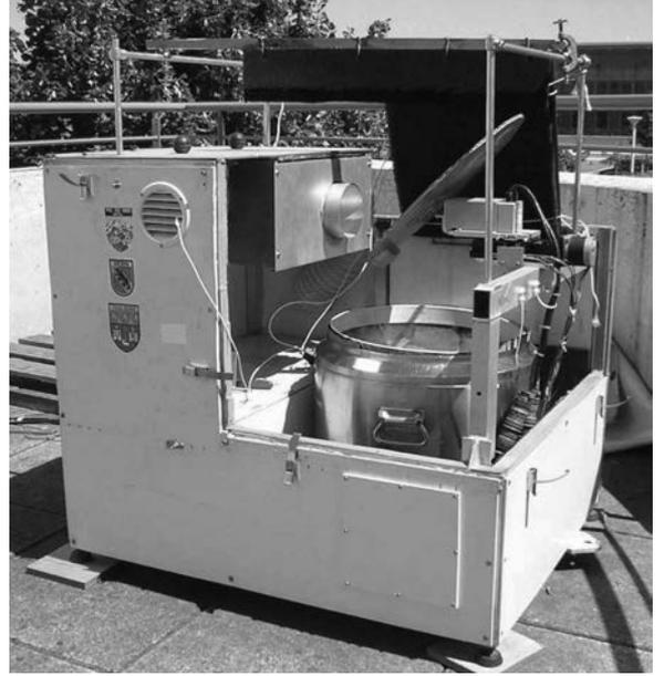
Fig. 1. MobRa instrument for the measurement of middle atmospheric H<sub>2</sub>O on the terrace of the Laboratoire d’Aérogologie, Toulouse, France.
