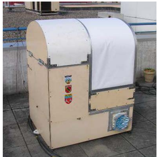
Fig. 1. The MobRa instrument for the measurement of stratospheric H 2 O on the terrace of the Laboratoire d'Aérologie, Toulouse, France.
